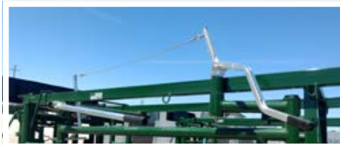
Head gate assist helps the rancher to close the headgate from further back down the chute. (not included with standard system)
