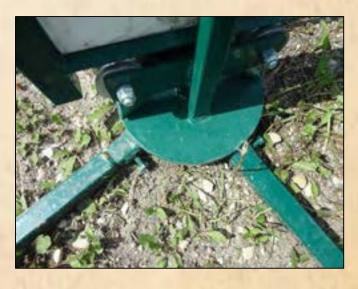
5. Insert both other ends into the center round plate of the swing door and tighten bolts.
