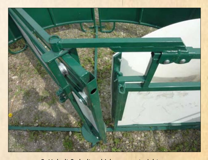
2. Unbolt 2x bolts which are on straight section of crowding tub. Slide along rail until cylinder piece slides over top of cylinder piece on the top of the swing n slide door. As per above picture. Firmly tighten bolts. Ensure door swings and slides freely around crowding tub.
